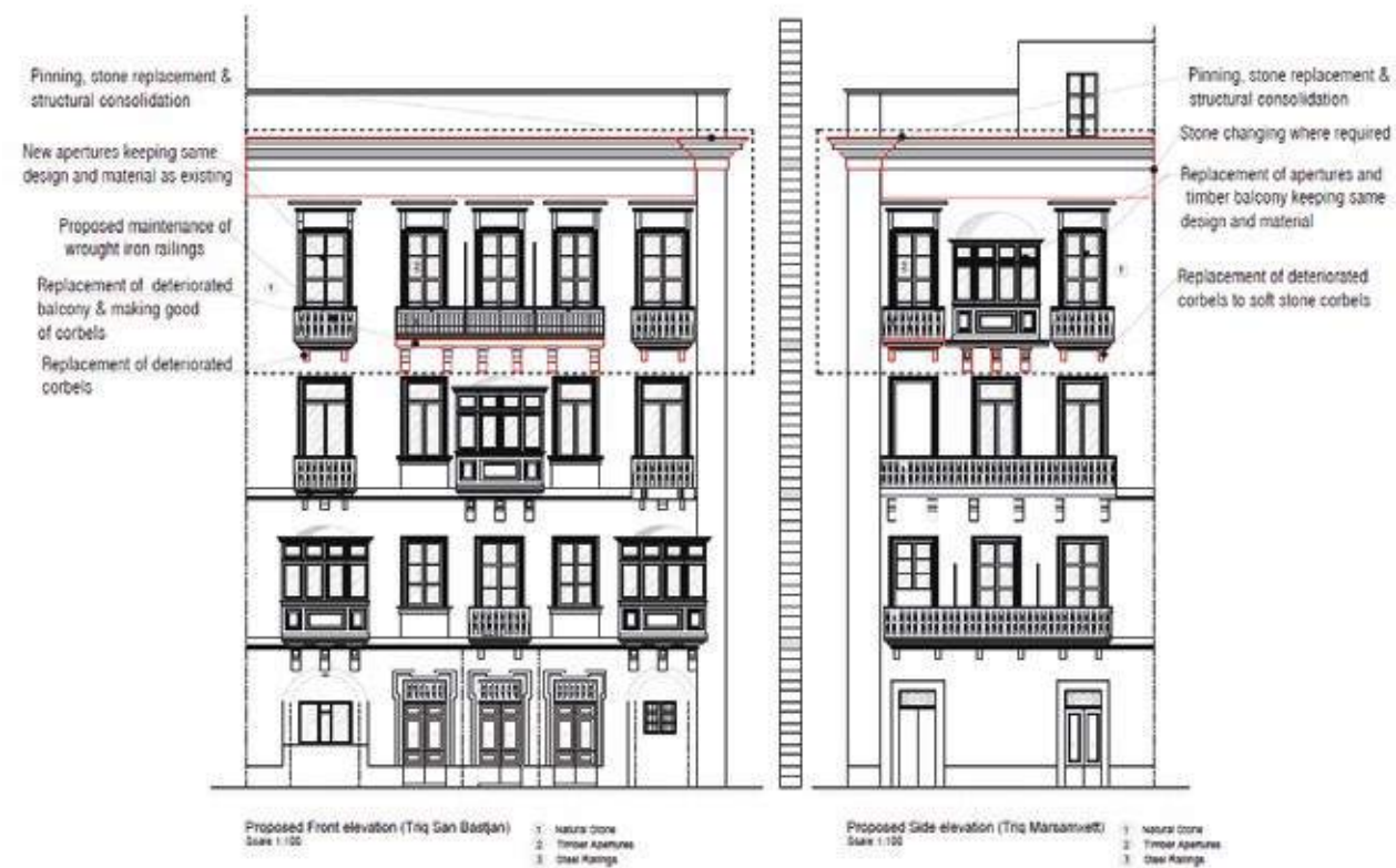
Structural Repairs on Façade - Valletta
