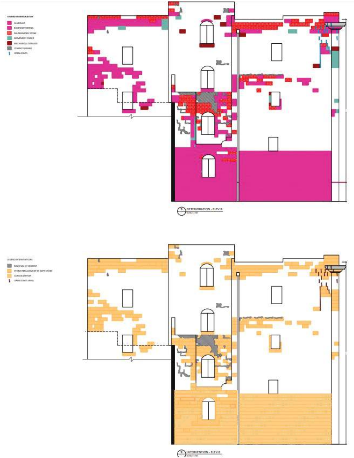
Restoration of Façade, Mapping of Materials – Cospicua
